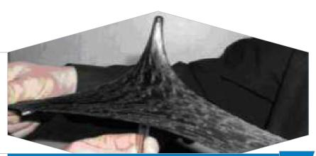
Polymer bitumen modification
